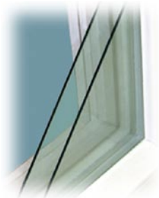
Single Strength Dual Pane LoE 3 Glass with Argon Fill
